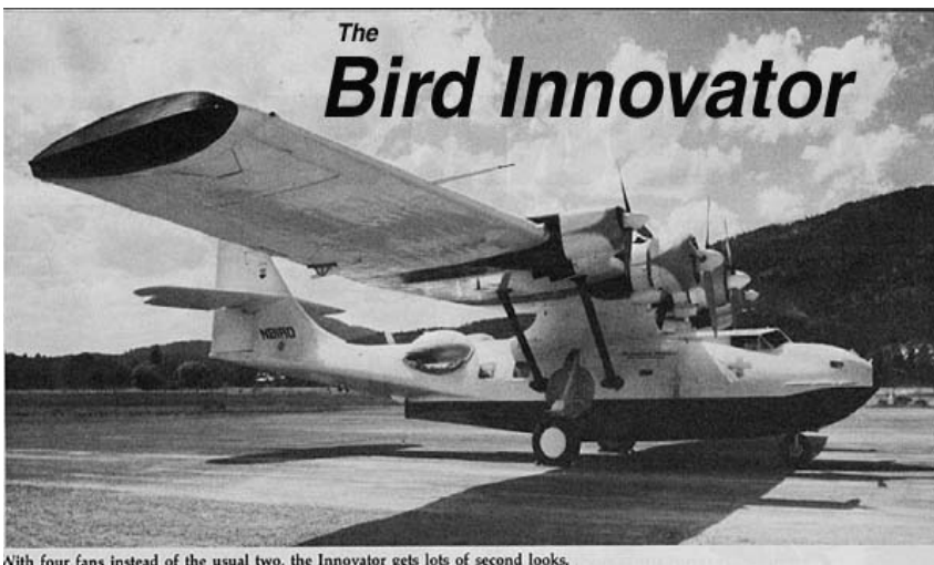
With four fans instead of the usual two, the Innovator gets lots of second looks.
